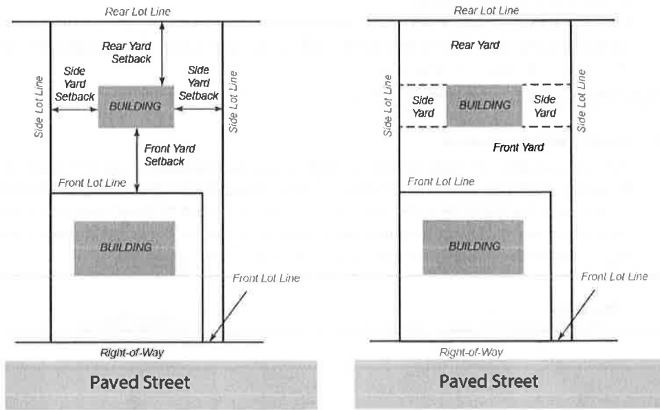
Figure 4.9-G: Typical lot lines and setback locations for a flag (panhandle) lot (left image) and typical yard locations (right image).
