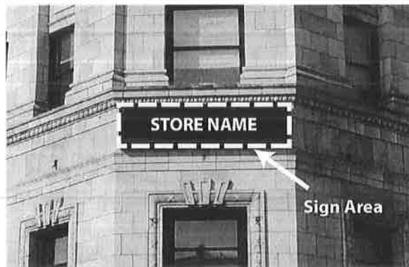
Figure 10.5-C: Illustration of computing the sign area for wall signs with a background panel or cabinet.
