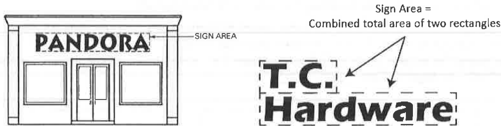
Figure 10.5-E: Illustration of sign area calculation for two differently shaped wall signs with individual letters.
