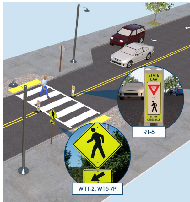
High-visibility crosswalk enhancements Source: FHWA
